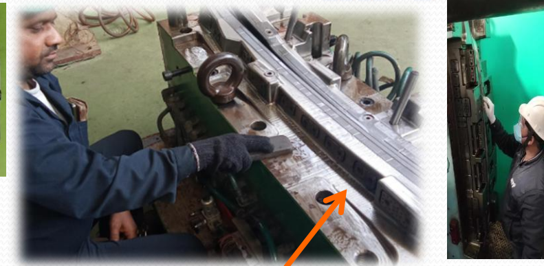
Air vent cleaning by tool room person
